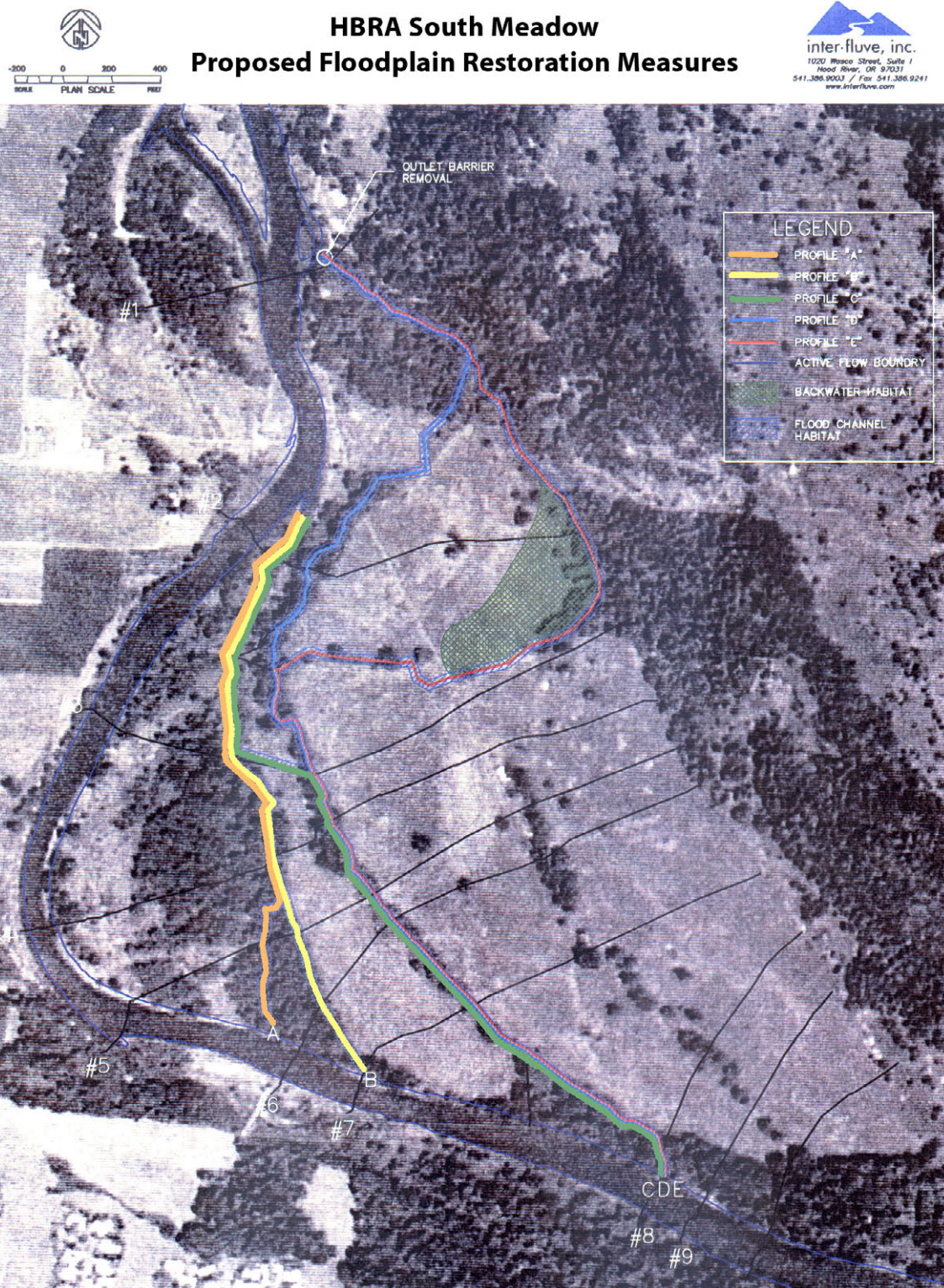
Figure 9. Proposed floodplain restoration measures, September 2002. Note channel letters at the south end of the South Meadow (Inter-fluve 2002).
